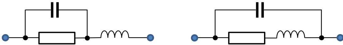
Figure 16.4 Possible equivalent networks for thin-film resistor
